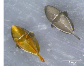
Fig. 1. Microrobot utilizing a functional coating. (Right) A bare magnetic microrobot made of thin assembled nickel pieces, based on [3]. (Left) A microrobot coated with an oxygen-sensitive film.
